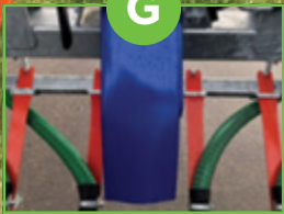
G Stone trap to easily remove any foreign objects from the Distributor
