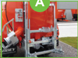
A Hydraulic mast to allow easier lowering while in the field and easier to detach Tri-App from the tanker
