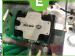
E Auto-reverse fitted as standard - distributor automatically reverses to prevent blockages
