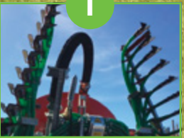
I 125mm (5") pipe at a 35 degree bend for rapid emptying of the tank
