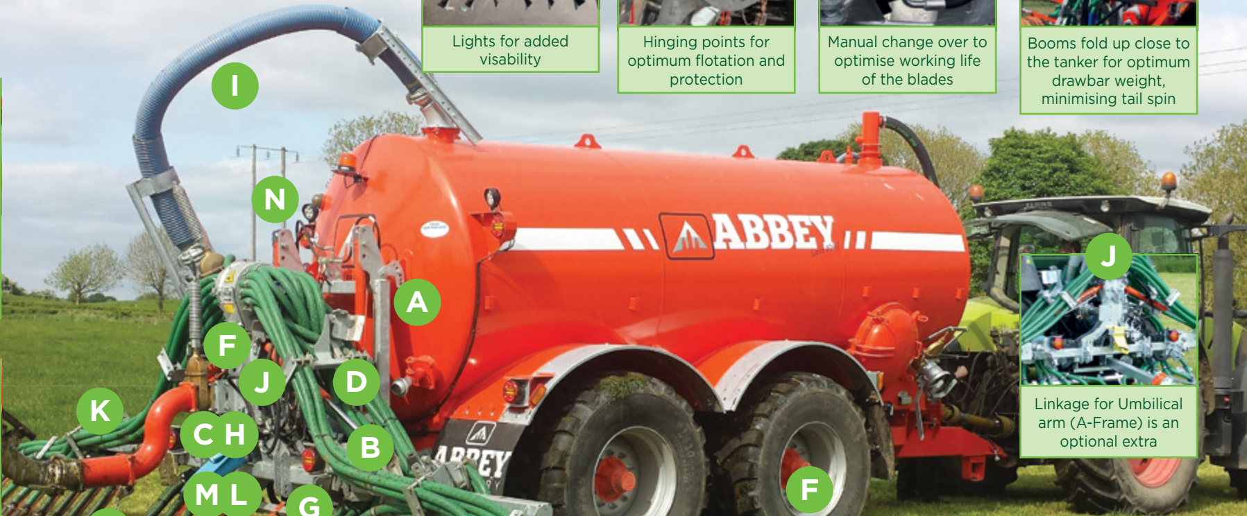
A Hydraulic mast to allow easier lowering while in the field and easier to detach Tri-App from the tanker
