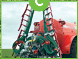
C Vertically folding booms for safe transport on the road
