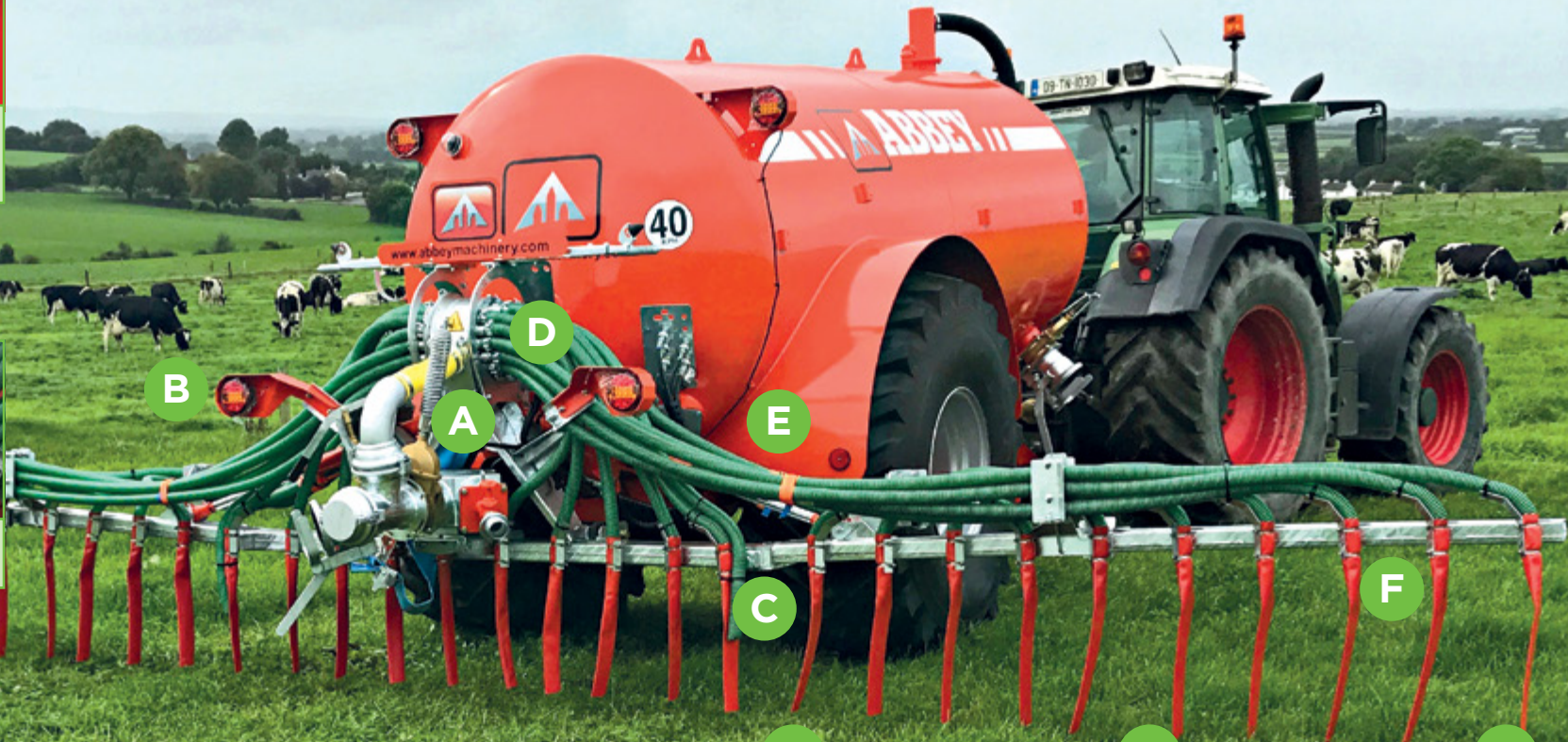
A Extensive brackets to support the applicator on the tanker
