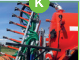
K Booms fold up close to the tanker for optimum drawbar weight, minimising tail spin
