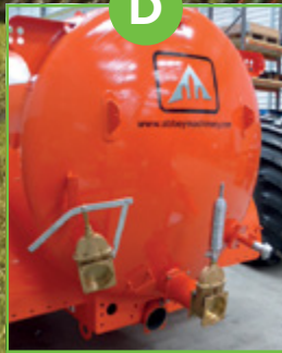
D Applicator ready brackets includes moving the rear access door to the side of tanker and stone trap
