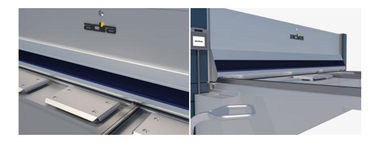
Possibility of retracting the back gauge at the end of the 1000-mm stroke
