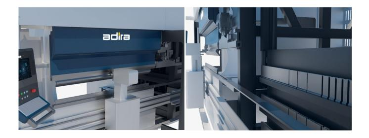
Manage the tools needed for bending. The system selects and positions the tools and dies available in the automatic tool warehouse, avoiding the manual selection and changing of tools and dies
