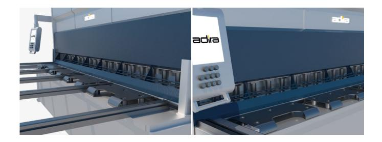
Robust back gauge with movable positioning, allows rotation for retraction of the guide
