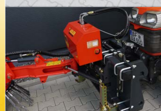
Universal attachment with side outward swivelling
