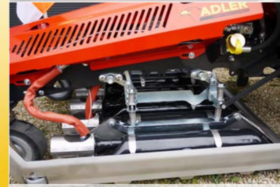
Spring-mounted infra box, height adjustable by radio remote control
