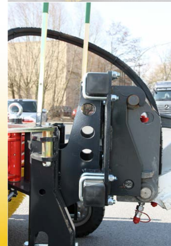
Wheel loader mount with castor guide and 3D levelling system
