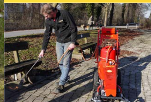
Hand-held burner for difficult-to-reach corners and edges
