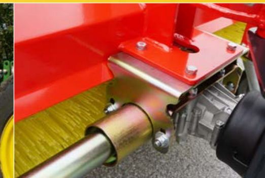
Brush speed and direction, and transmission position are adjustable
