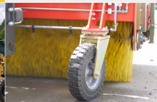
Three large swivel castors 400 mm x 100 mm
