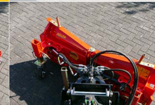
Farm loader attachment with levelling system and parking support
