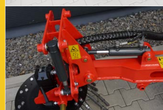
Hydraulically adjustable longitudinal and lateral inclination (mechanical/hydraulic)
