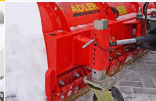
Height-adjustable support wheels (200 x 80 mm)
