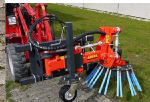
Swivel arm (mechanical/hydraulic) to work on large surfaces
