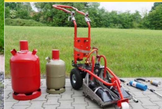
The Flexi can be operated with an 11-kg or 5-kg gas cylinder. Refillable gas cylinders and disposable cartridges are available for use with the hand-held torch.
