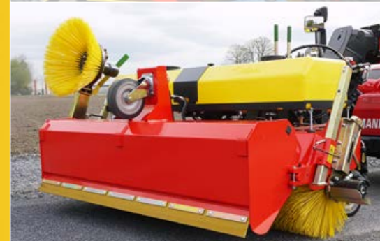
Simple sweeping mode, hydraulic hopper emptying system and third support wheel on hopper
