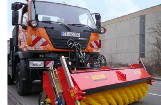
Unimog fitting with attachment mount as per DIN 76060
