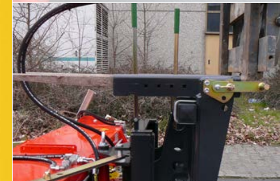
Wheel loader mount for fork prongs with castor guide and 3D levelling system
