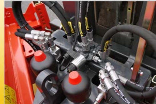
Electric switch valve with overload protection provided by two pressure relief valves and nitrogen bladder accumulator
