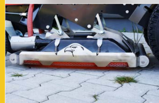
Height-adjustable infra box to adapt to road, path and surface conditions
