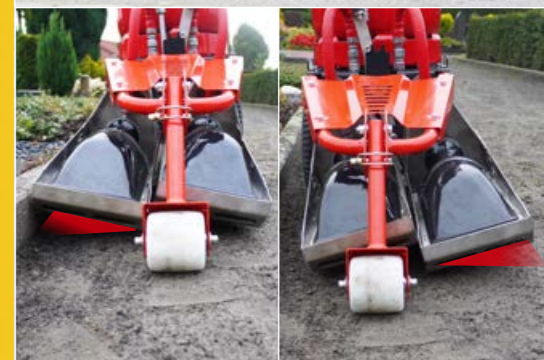
Ideal for treating edges by simply tilting the emitter to the right or left.
