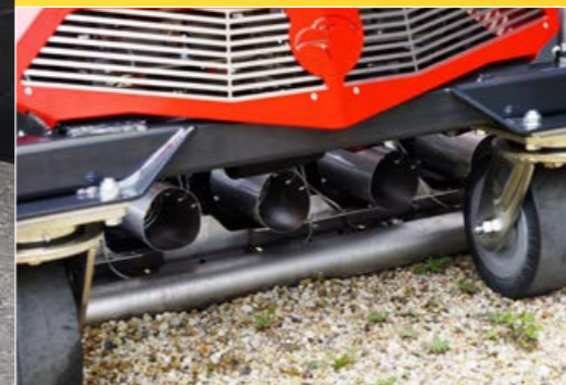
Impact-absorbing and heavy-duty swivel castors to protect infra box
