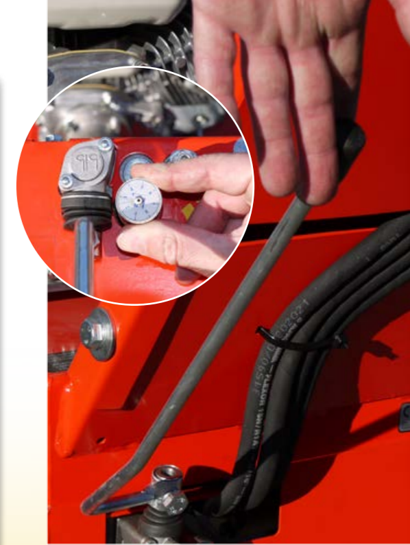
Hydraulic rod steering system and continuously adjustable traction drive
