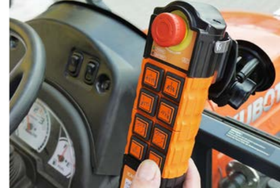
Radio remote operation for convenient control in the cab
