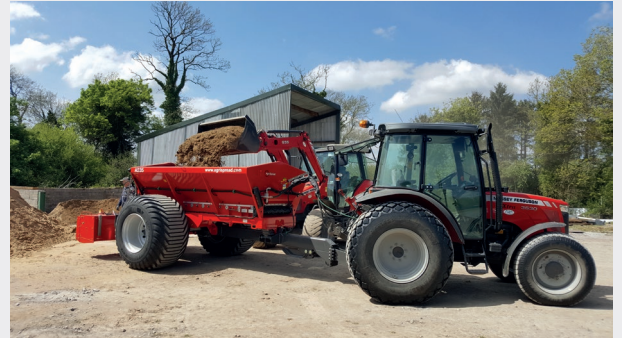
AS35 Combi-Spread being loaded with sand, Peat and soil mix for divot repair
