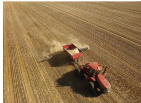
AS130-T with wind booms spreading lime sand in Western Australia
