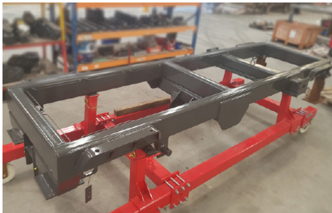
Chassis entering the assembly line on a mobile trolley
