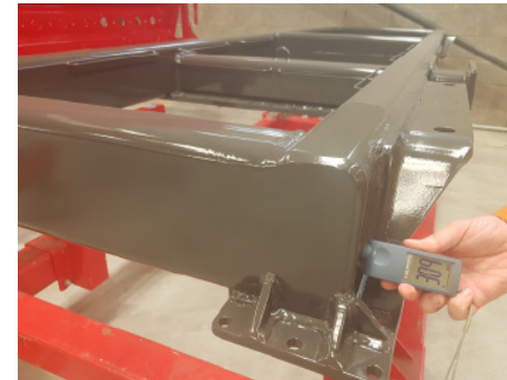
Chassis being checked in quality control for paint thickness and hardness
