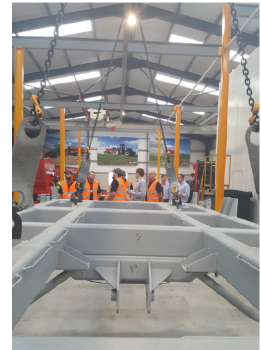
chassis on overhead line
