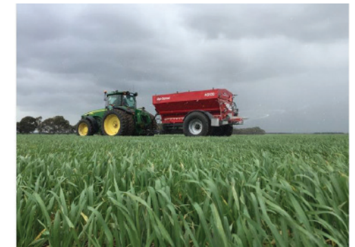
Spreading urea at 36m at 120kg/ha
