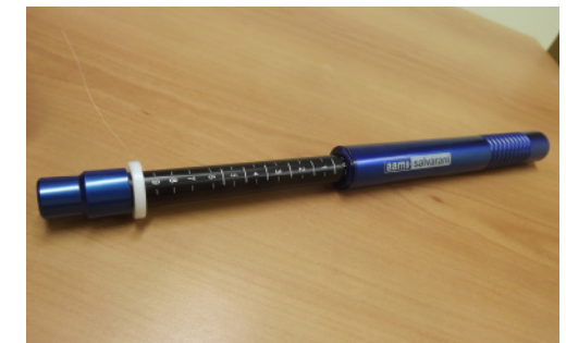
Hardness tester: Very important to check the fertiliser has the required strength to spread at wide widths
