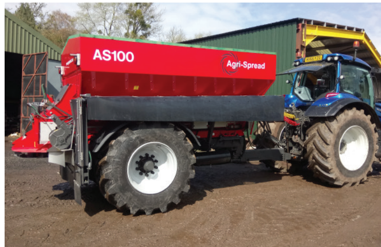
AS100 hydraulic drive with wind booms fitted. The hydraulic drive floor is controlled via GPS and a Rate controller. Stand alone rate control monitor or ISOBUS systems available.
