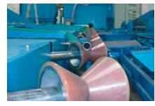
Diabolo blast machine for handling sprinkler pipes
