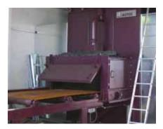
Blast machine for metal sheets
