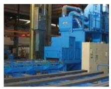
Blast machine with adjustable passage height
