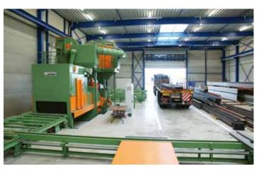
Crossover conveyors connect the roller conveyor blast machine with the sawing and drilling machines.
