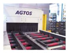
Blasting machine with adjustable passage height
