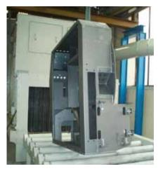
Blast machine for metal sheets, sections and constructions with a passage height of up to 1000 mm
