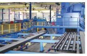
Blast machine with crossover conveyors
