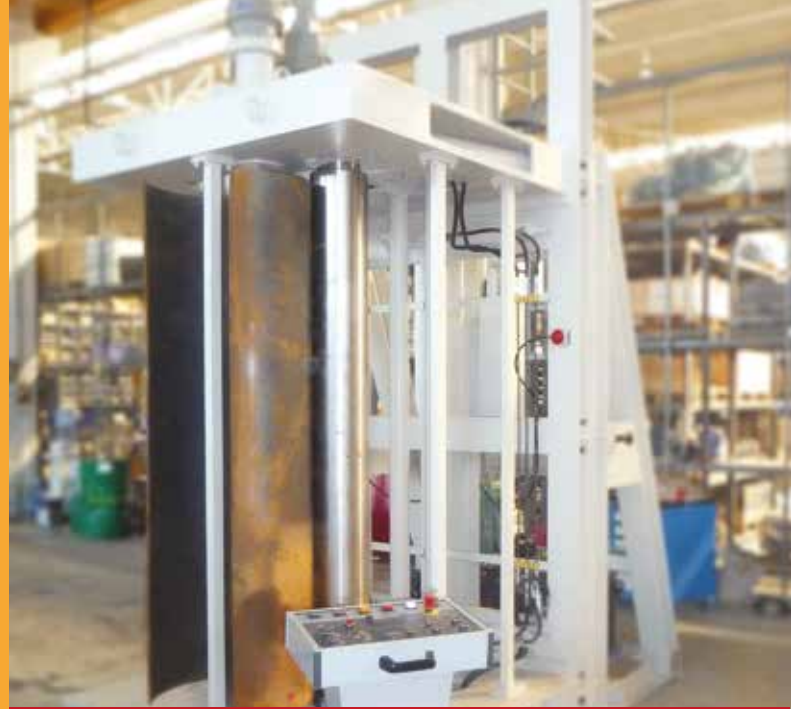
Ahs 4 rolls vertical plate bending machine Ahs 4 valsli dikey silindir makinesi
