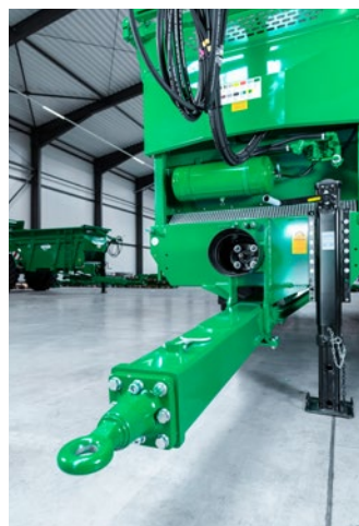
Picture left: The series standard lower coupling with 50 mm ring hitch. The vehicle components are protected by a cover from external influences.
