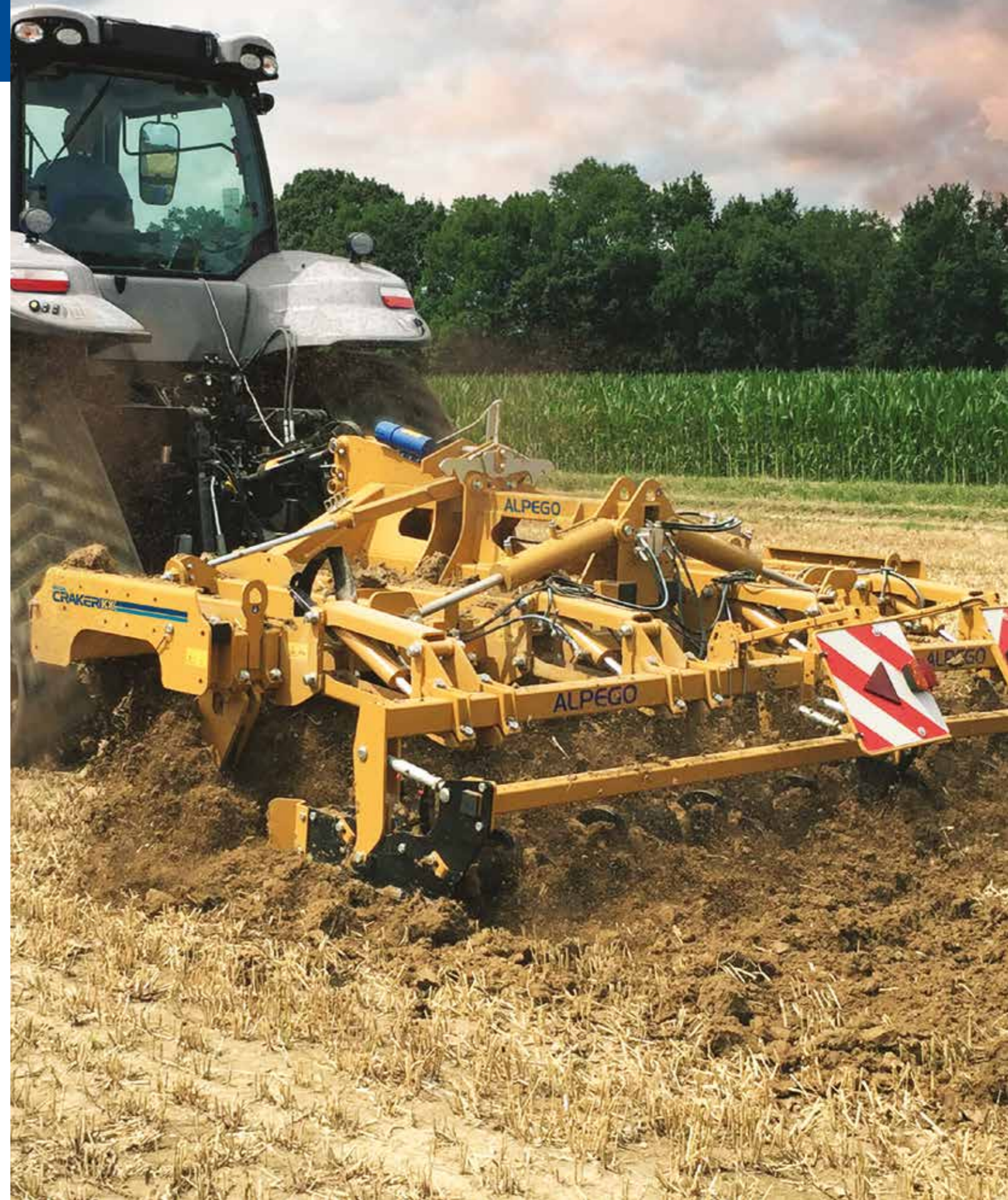
HYDRAULIC CIRCUIT Mega Craker KX subsoilers are equipped with roller with parallelogram system using a working depth control with a cross hydraulic circuit.
