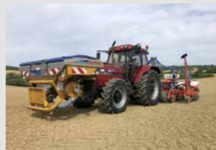
Fertidrill AS-PRO with precision seed-drill
