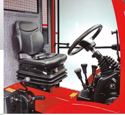
The adjustable steering wheel allows any operator to find his ideal driving position. On the left of the driver's seat there is a large glove compartment with a soft rest that is very useful for storing the operator's things and tools.
