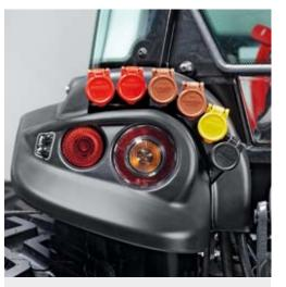
Hydraulic system with 3 distributors: 1 double effect, 1 double effect with floating position with static lever, 1 simple effect + oil flow outlet. Total: 6 rear quick release catches.
