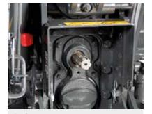
PTO • Gearbox with PTO 540-1000 rpm • Gearbox with PTO 540-5405 rpm
