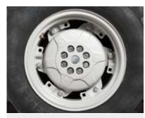
REAR CAST IRON WHEEL FLANGES Flanges that increase the weight of the tractor at the rear.
