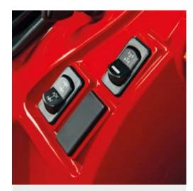
The rear differential lock prevents slipping and optimizes traction. The front traction disengagement is useful when travelling along roads and prevents damage from being done to delicate grounds.
