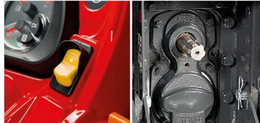
The two speed PTO: 540/540E rpm as standard, 540/540S rpm, 540/1000 rpm\* and synchronised with the gearbox speed. The ASAE 1 3/8 PTO shaft is the same for all speeds.
