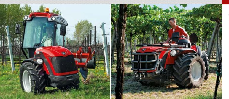
The short wheelbase and tight steering radius make the tractor extremely agile in crop rows. The smooth and sensitive hydroguide steering wheel assures precise maneuvering on steep slopes, in crossways movements, in narrow paths, among crop rows and in car parks. The hydraulic system of the hydroguide uses the Load Sensing system to obtain a constant flow of manoeuvrability independent of steering speed.
