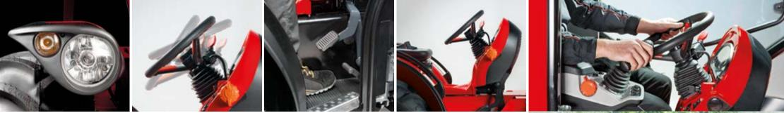
The lighting equipment, integrated into the mudguards, is comprised of reflecting parabolic optical assemblies, which offer a wide range of illumination covering the roadway, the equipment, and the surrounding field. The adjustablesteering wheel allows any operator to find his ideal driving position. Maintenance is practical and fast thanks to the fact that the bonnet can be fully opened and the side panels and battery cover can be easily removed.
