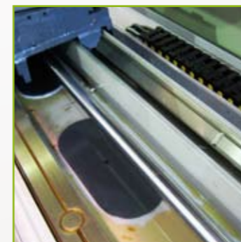
LUBRICATION Forced lubrication of slide ways
