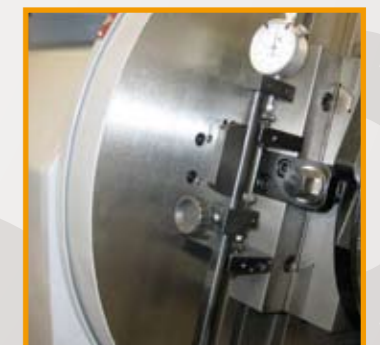
Stroke comparator reduces journal set-up time
