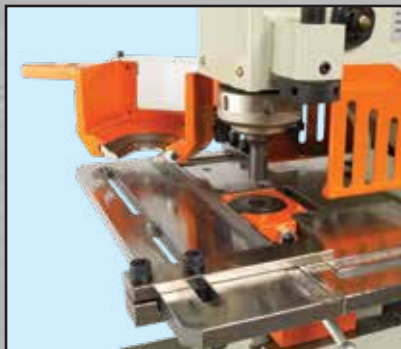
Swing away stripper for easy access and fast tooling changes.
