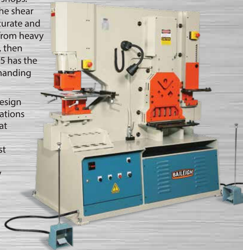
Shearing station with hydraulic hold down
