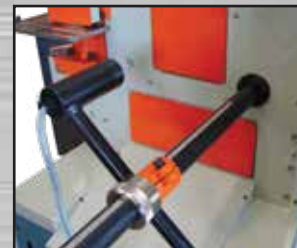
Electric back gauge
