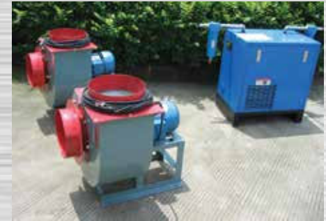
Exhaust and air dryer
