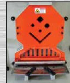
Shearing station with hydraulic hold down
