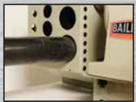
3. Reinsert Pipe to Notch Opposite Side
