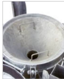
Funnel with filling pipe
