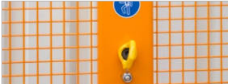
PPE anchor point (personal protective equipment)
