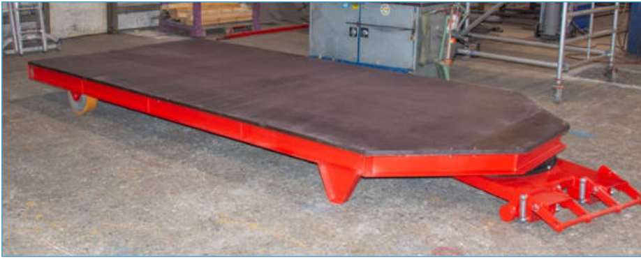
STS with anti-slip "Betosieb" boards
