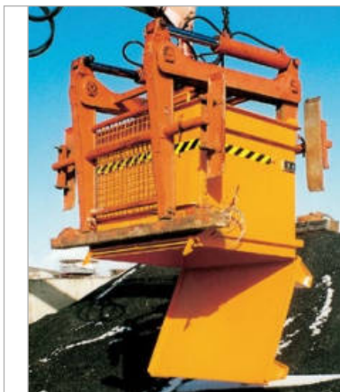
BC with brick clamp operated trap door
