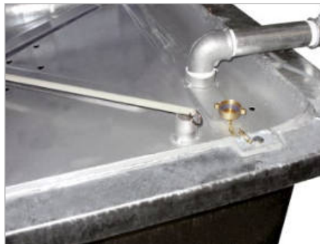
Dipstick to control the fill level
