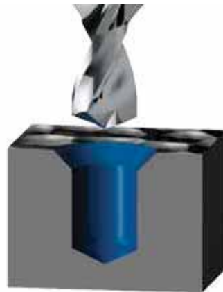
Pilot Hole Drilling
