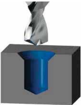
Pilot Hole Drilling
