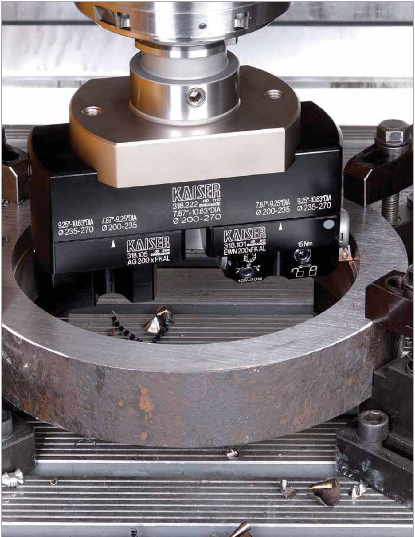
B.4 LARGE DIAMETER BORING
