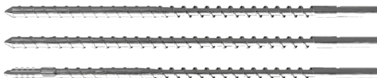
Screw examples (top down): 4:1 metering screw, 4:1 core progressive screw, 4:1 dispersion screw with Maddock and mixing segment
