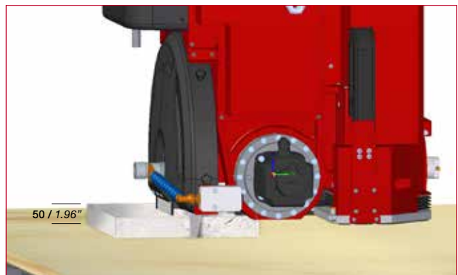
Spessore max. lavorabile con \varnothing disco 350mm Max. workable thickness with \varnothing 13.8" saw blade
