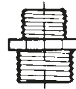
Nipple, reduced, with outer thread.
