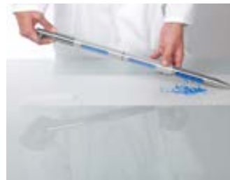
Sealing sleeves zone sampler 25 mm usage
