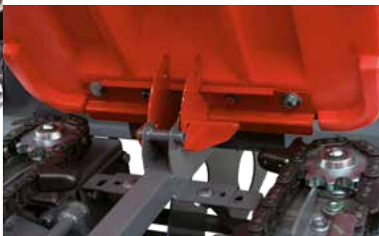
The hood can be dismantled without special tools, making maintenance of the header convenient and easy.
