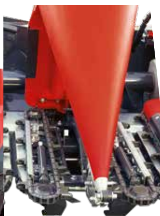
The hood can be dismantled without special tools, making maintenance of the header convenient and easy.
