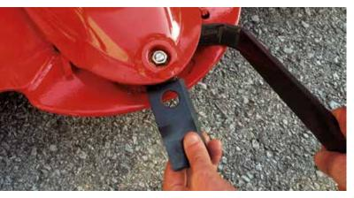
Quick-change knives dramatically reduce replacement time without the use of tools. Cutting discs are made to have a remarkably close proximity of knives and provide a perfect cut even with packed and wet product.
