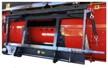
The fluctuating adapter plate enables the header to contour to the terrain. SPARTAN is adaptable to all kinds and models of forage harvester with a simple replacement of the adapter kit.
