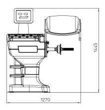
Available in two versions: Manual locking, electric brake (ER80) Pneumatic locking with safety control and electric brake. (ER80SE)
