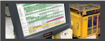
Monitors and keeps a record for all machine runtimes, production schedules and maintenance which is viewable and controllable online. This program runs on 2 super computers that are connected to the Internet. It allows problem solving with help of engineers and experts sitting anywhere in the world in a matter of minutes.
