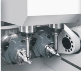
The multiplier effect – more spindles, more cutting, more profit: The combination of 2 spindles and a 4-fold clamping device results in a cost saving of up to 50%. Doubled productivity on one machine means a reduction of machining time of nearly 50%. There is also the option of multi-side machining through NC controlled rotary axis.
