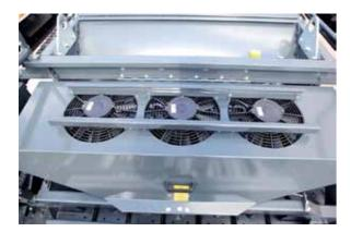
Our Big Balers are equipped with high performance fans and powerful nozzles blowing at adjustable intervals (optional) in order to ensure a stable cleaning of the knotter area under any condition. High effective cleaning system assures to operate in total security avoiding control stoppages and additional cleaning operations.
