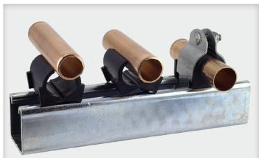
**CUSH-A-CLAMP** — Channel mounted clamping systems are ideal for multiple line runs, while absorbing shock and vibration, reducing unwanted noise, and preventing galvanic corrosion. Cush-A-Clamp fits any standard 41mm (1-5/8") wide channel.
