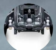
**Ball-head coupling** The K80 ball-head coupling is ideal for heavy-duty trailer operation. It is retractable, height-adjustable and can be removed to make the PTO more accessible. The K80 can absorb a theoretical thrust load of up to 4 tons, thereby utilising the load capacity of wheels and rear axle to an optimum level.
