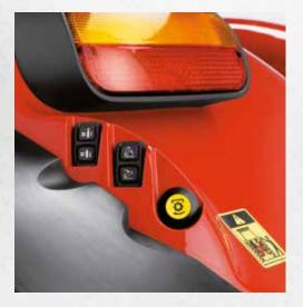
External actuation for rear PTO, rear hitch and a control unit for each of the rear mudguards.
