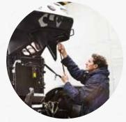
One-section bonnet support by gas struts can be lifted into two positions  $(45^{\circ}/90^{\circ})$ , even with a front-mounted attachment.
