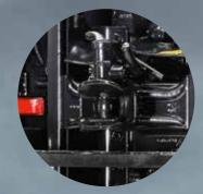
**Automatic trailer drawbar** Is individually adjustable for height and the towbar coupling is opened by remote control from the cab.
