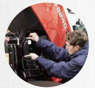
Continuous cleaning via a Piclon filter ensures that the filter only needs to be maintained when the corresponding warning lamp lights up.
