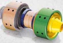
Continuously variable transmission from 0 to 50 km/h.
