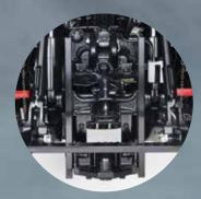
Wider trailer carriage The trailer carriage for the towbar coupling being used is now wider and this makes it easier to connect up the universal shaft to the PTO stub shaft. The new modular design also makes it easy to retrofit a K80 ball-head coupling.
