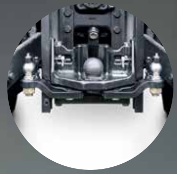
Ball-head coupling The K80 ball-head coupling is ideal for heavy-duty trailer operation. It is retractable, height-adjustable and can be removed to make the PTO shaft more accessible. The K80 can absorb a thrust load of up to 4 tons, thereby utilising the load capacity of wheels and rear axle to an optimum level.
