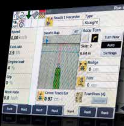
S-Turn II turns automatically at the end of a tramline
