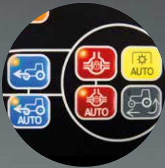
Automatic all-wheel drive and differential lock management
