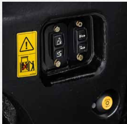
Easy to reach: External actuation of front hitch, front PTO and front control unit.
