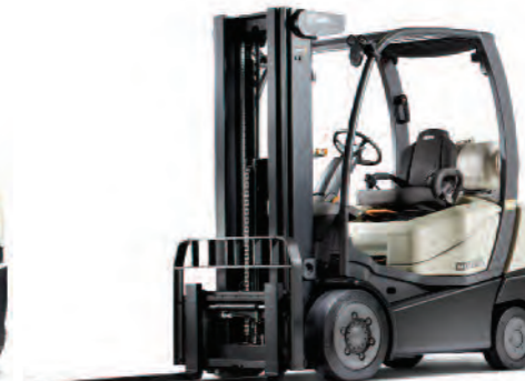
C-5 Series 4-Wheel LPG Counterbalanced Truck with Cushion tyres Load Capacity: 2000 and 3000 kg Lift Height: 2920 to 7465 mm
