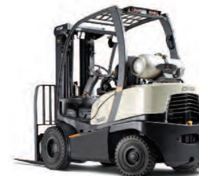
C-5 Series 4-Wheel LPG Counterbalanced Truck with Super Elastic tyres Load Capacity: 2000 and 3000 kg Lift Height: 2920 to 7465 mm
