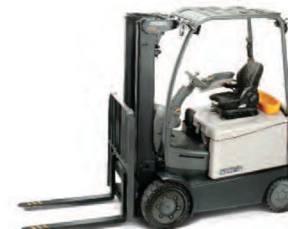
FC 5200 Series 4-Wheel Counterbalanced Truck Load Capacity: 2000, 2500 and 3000 kg Lift Height: 3200 to 7925 mm
