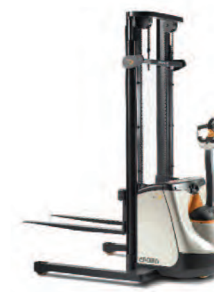
ST 3000 Series Straddle Stacker Load Capacity: 1000 kg Lift Height: 2400 to 4250 mm
