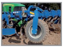
The implement is supported by 2 wheels. The mechanical depth adjustment is easily achieved.
