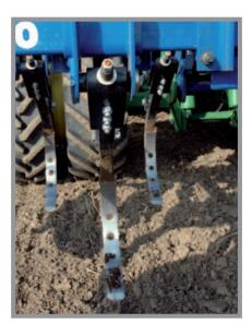
The implement is mounted with the new developed 2-D tine, which turns 20 cm horizontal and 30 cm vertical.
