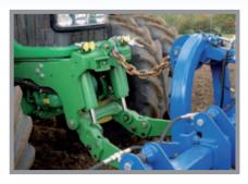
To achieve a precise working depth the Cultivator is mounted with a chain instead of a top link. The flexible chain makes the implement work freely via the carrying wheels and the front linkage.
