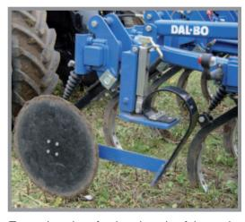
To avoid a ridge of soil to the side of the machine spring loaded discs are mounted on either side. The Discs can be adjusted in height by the turn of a spindle.
