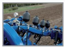
The **FrontCultivator** comes as standard with hydraulic stone protection. This provides huge advantages and ensures efficient work even under the most difficult conditions.
