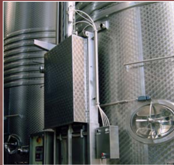
PNEUMATIC GUILLOTINE HATCH
