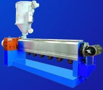
Kablo-Tel plastik izolasyon extruder Cable – Wire plastic insulation extruder
