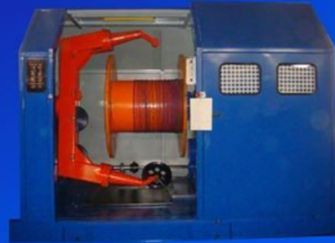
Bantlı çekici-itici –verici makina Capstans - pusher – transmitter machine
