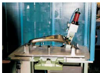
Device for Ø8 holes in sheet metal
