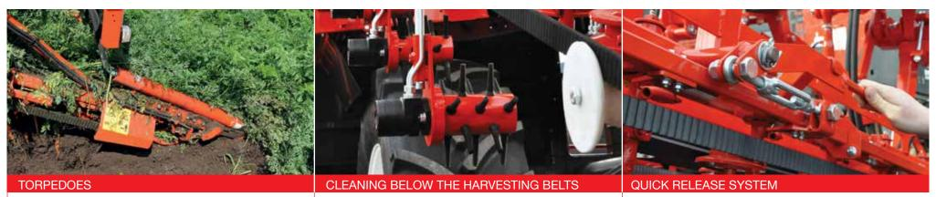
The 2 hydraulically driven rotary torpedoes per harvesting element ensure an accurate intake of the haulm. If you, as a driver, want to concentrate better on the actual harvesting process, you can opt for DAS (Dewulf Automatic Steering). ADC (Automatic Depth Control) is standard.
