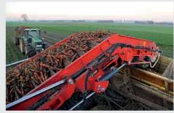
higher on the chassis. The product is therefore transported up at a significantly lower angle, ensuring that no product falls back. Combined with a large drive sprocket on the end, a highly product-friendly transport can be realised under all conditions.
