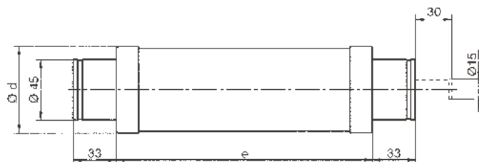
Fig. 2 Dimensions acc. to DIN 43 625 in mm
