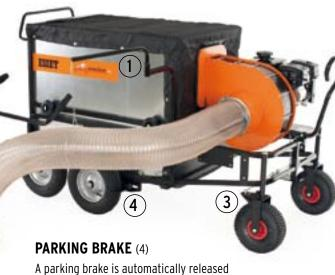
when the machine is moved forward.
