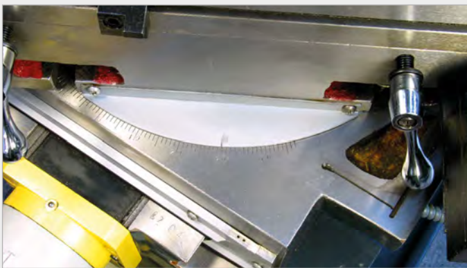
cross table rotatable 45° to the left and 45° to the right.
