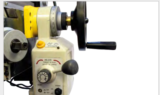
Y-axis with stepless feed control
