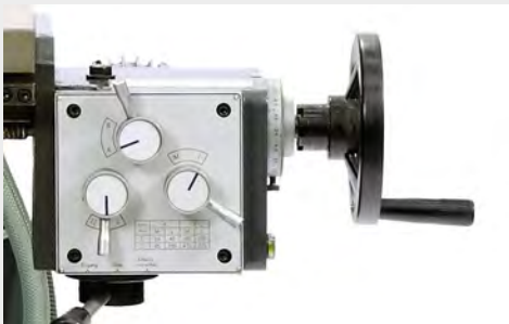
Automatic feed for the X-axis as standard (8 speeds)
