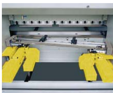
Sechs-Achsen Hinteranschlag (X1-X2-R1-R2-Z1-Z2) / Six axes backgauge (X1-X2-R1-R2-Z1-Z2)
