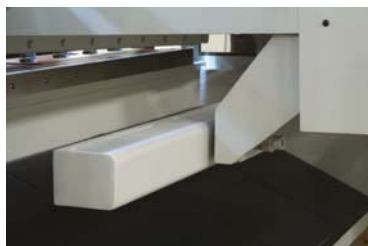
Hinteranschlag-Schwenk-System / Swing-up backgauge system
