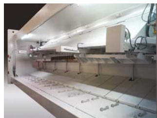
Anti-Verdrehsystem (optional) / Anti twisting system (optional)
