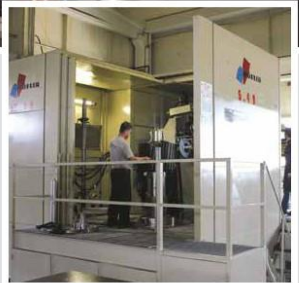
CNC Gear Grinding Machine up to 2500 mm diameter and 35 modules
