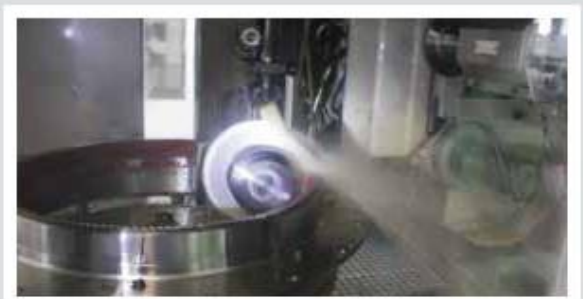
CNC Gear Grinding Machine up to 2500 mm diameter and 35 modules
