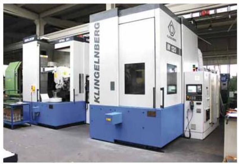
1200 mm CNC Gear Profile Grinding / CNC Profile Measurement and Interior Gear Profile Grinding
