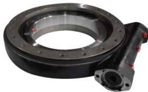
TOWER ROTATION REDUCER ER528 i:1/102 TORQUE NM 4500 POWER 0,47 KW
