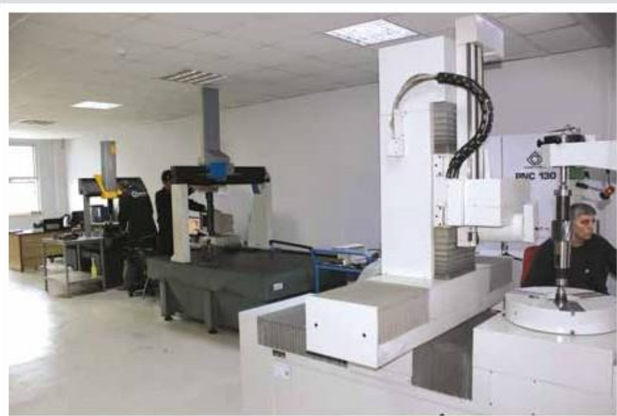
1200 mm CNC Gear Profile Grinding / CNC Profile Measurement and Interior Gear Profile Grinding
