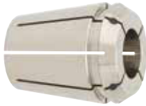
Tap Collets GERC-GBD with Internal Square Drive and Seals for IC (Inner Coolant Supply) – 10µm
