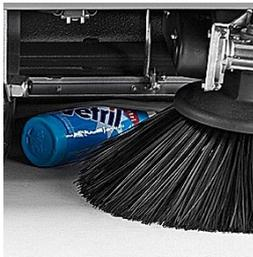
The flap fitted to the front of the machine is activated from the driver's position and allows the main brush to pick up bulkier debris
