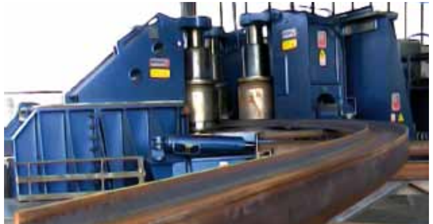
Variable Geometry Beam and Section Benders with capacities up to section modulus 17.000 cubic centimetres.
