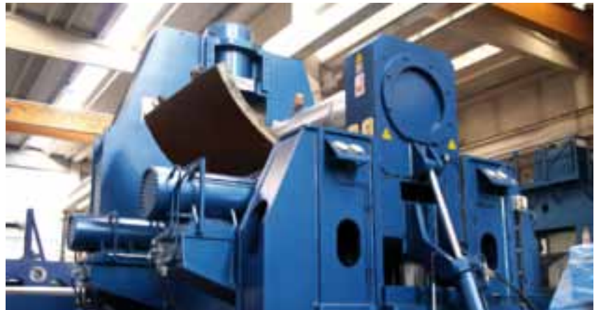
The highest rolling capacities (3500x280 in cold conditions) have been achieved in 2009 with the model HAV 15/S.
