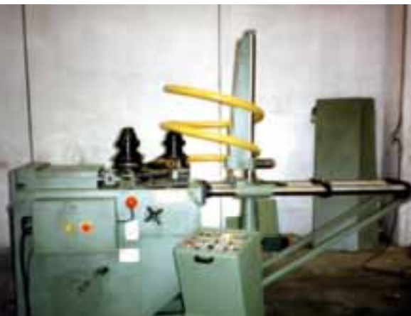
Spiral Rolling equipment and Spiral Supports for medium and heavy duty applications.
