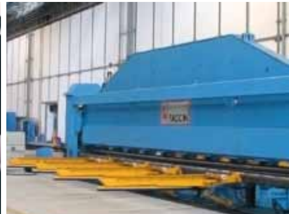
Roll Presses for aerospace and shipbuilding applications up to 21 meters plate width.
