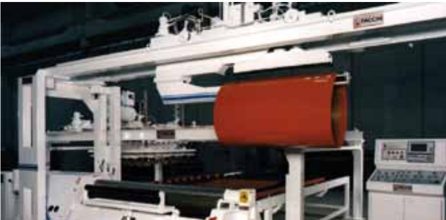
Integrated Loaders, Feeders and Ejectors for complete automation of the rolling cycle. Ideal for the production of HVAC components.
