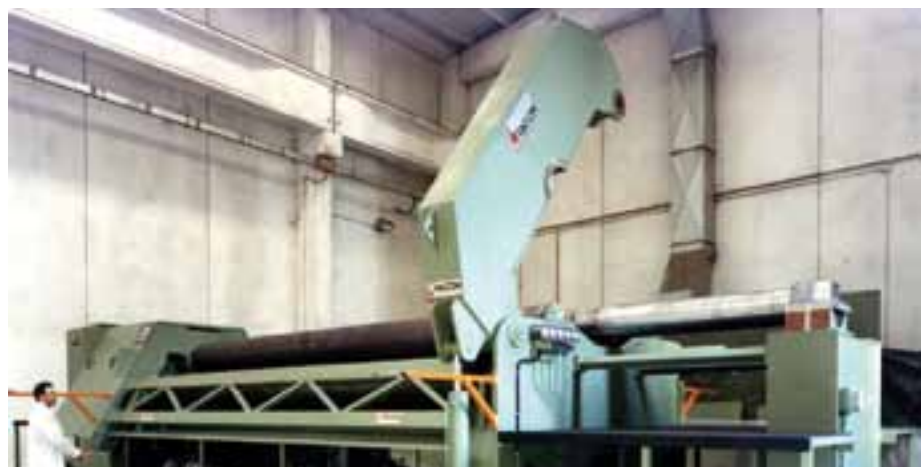
Special versions of four and three roll machines with preloaded top rolls for rolling thick walled long pipes (Oil & Gas Pipelines).
