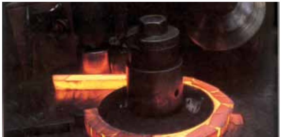
Rotating Table Ring Rolling Machines, ideal for flat and angle bars used as flanges and bearing housings. Capacities up to 70.000 square mm cross-section.
