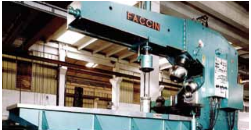
Automatic Flanging Machines are available in different design for heads with or without centre hole. Playback CNC controls are also available.
