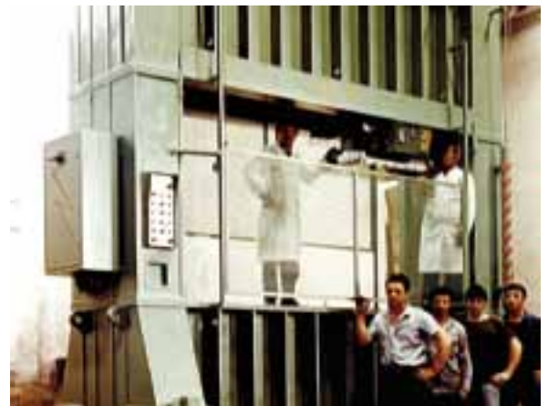
Hydraulic Presses are also designed specifically with movable tools for roll bending or straightening of plates. They are dedicated to general fabricators or shipbuilders.
