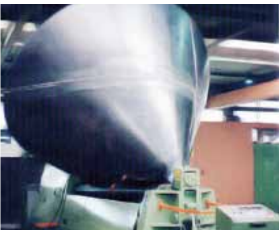
Conical Rolls Verions for automated cone rolling lines (for cement mixers or for the food processing industry).
