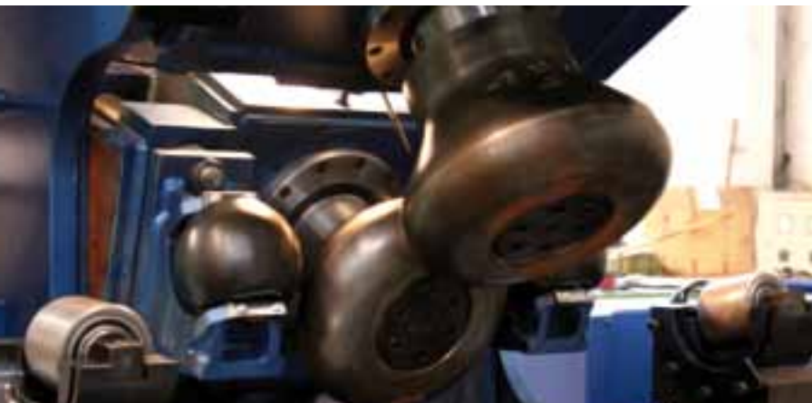
Dedicated Solutions are provided to optimize productivity, precision and ease of use in flanging of mild and stainless steel heads in any size and shape.
