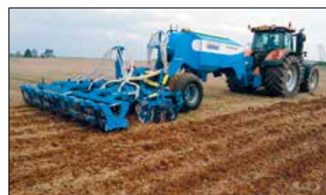
Mounted cultivator for strip-till soil cultivation.
