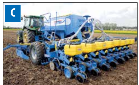
Precision sowing of corn and fertilizer application.
