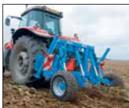
1. Ploughshares in one row for deep cultivation up to the depth of 60 cm.
