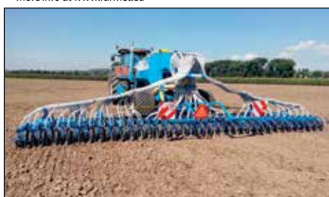
Wide seeding bar for sowing close-drilled crops.
