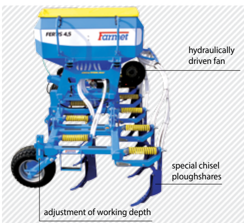
1. Chisel ploughshares for additional fertilization and cultivation in two rows. (Optional ploughshares, page 31).
