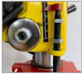
Graduated rod for drilling depth adjustment
