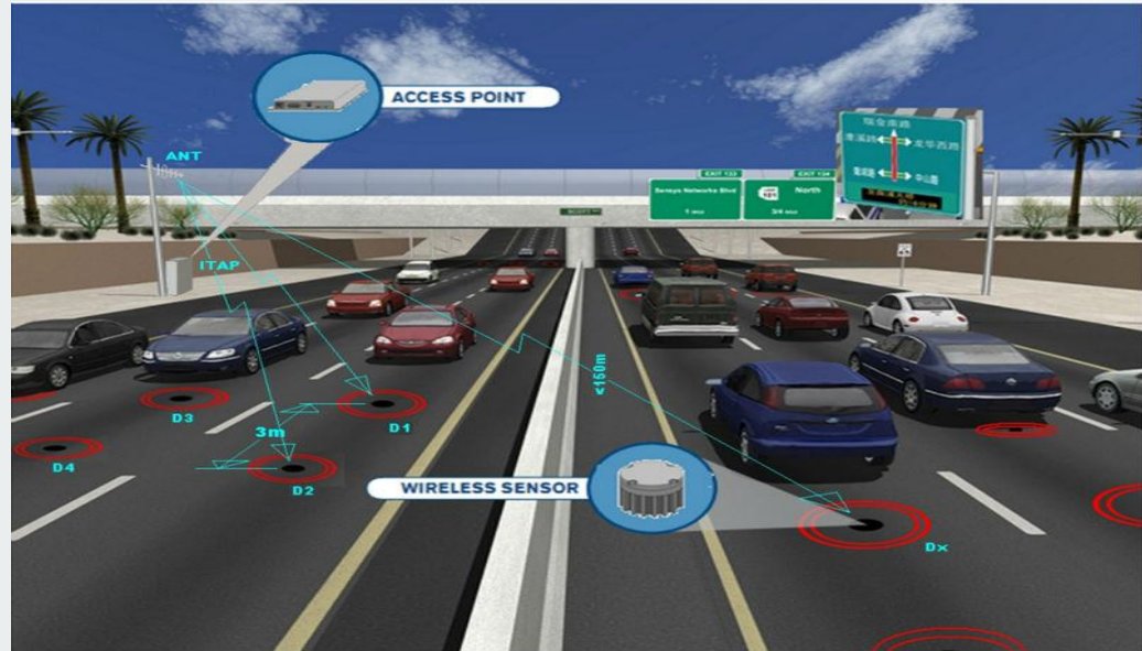
Highway Traffic Density and Speed management
