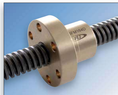
Colerette ronde Bronze CC493K (CuSn7ZnPb) selon ISO2901/2903 et DIN 103 tolérance 7H
