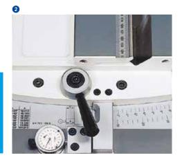
These axes achieve high process speeds, on the one hand, while on the other hand the short auxiliary times also guarantee maximum precision with in-feed movements of 0.0001 mm (0.000,040"). These axes can be equipped with rotative or linear measuring systems, depending on requirements.
