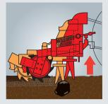
Suspended gear housing The stone protection spring operates as a saftey device against obstacles (option)
