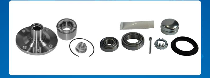
Flanges get axial run-out due to thermal loads which leads to brake judder. As the workshop needs to disassemble the flange and bearing, repair kits allow to renew the flange during wheel bearing repair without extra work.
